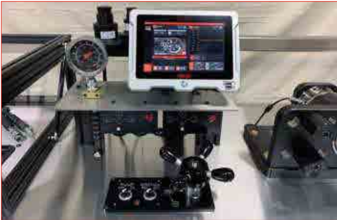
T-Box™ 2 at the centre of a test bench for hydraulic torque wrenches
