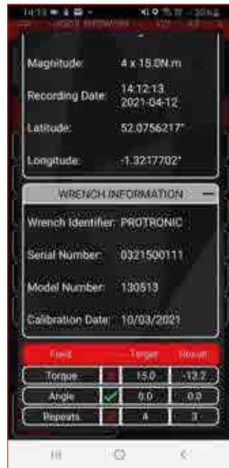
Application and tool information provides a comprehensive record for traceability purposes
